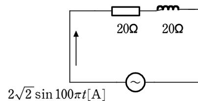
$$V = \sqrt{R^2 + \omega^2 L^2} I_0 \sin(\omega t + \phi)$$
