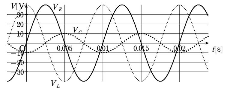
$$\begin{aligned} \text{⑩ } V &= V_R + V_L + V_C = 40 \sin 100\pi t + 40 \cos 100\pi t - 10 \cos 100\pi t \\ &= 40 \sin 100\pi t + 30 \cos 100\pi t \\ &= 50 \sin(100\pi t + \phi) \quad \tan \phi = \frac{3}{4} \end{aligned}$$
