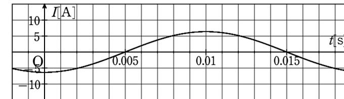
⑦  $P = IV = -\frac{V_0}{\omega L} \cos \omega t V_0 \sin \omega t = -\frac{V_0^2}{\omega L} \sin \omega t \cos \omega t = -\frac{V_0^2}{2\omega L} \sin 2\omega t$
