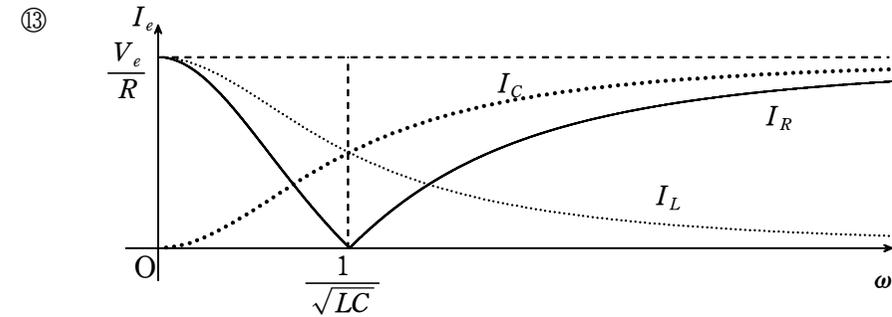
$$\omega = 0 \text{ で } I_R = I_L = \frac{V_e}{R}, \quad I_C = 0$$
