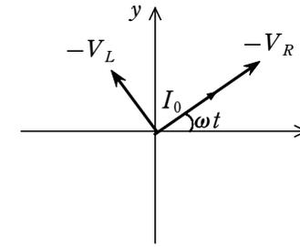
$$\begin{aligned} \text{④ } V &= RI_0 \sin \omega t + \omega LI_0 \sin\left(\omega t + \frac{\pi}{2}\right) \\ &= RI_0 \sin \omega t + \omega LI_0 \cos \omega t \\ &= \sqrt{R^2 + (\omega L)^2} I_0 \sin(\omega t + \phi) \quad \tan \phi = \frac{\omega L}{R} \end{aligned}$$
